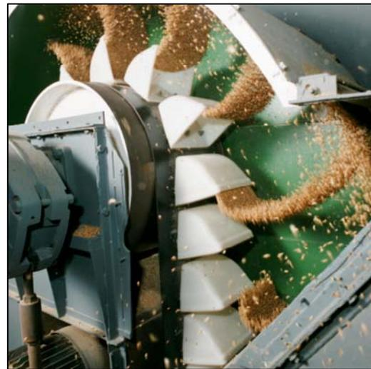
Centrifugal Discharge of CC-S Buckets
